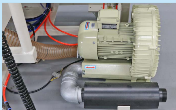
真空泵抽濕定位 Vacuum pump for vacuuming and fabric positioning
